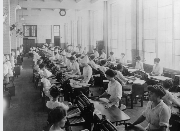
Workers perforating postage stamps at the Bureau of Engraving and Printing in 1914. The factory, with 146 machines, could produce up to 105,000 sheets of stamps daily.
